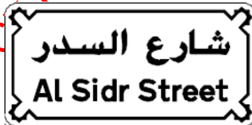
Figure 4: Typical Major Street Road Name Sign
