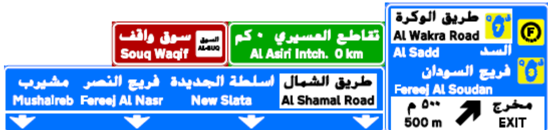
Figure 8: A Typical Advanced Direction Signs before an Interchange Exit
