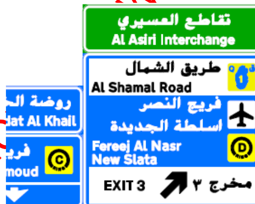
Figure 7: Typical Direction Sign at an Interchange Exit
