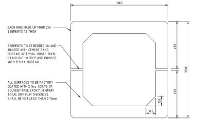
DETAIL OF PRECAST CONCRETE GRADE SRC 50 FIBRE REINFORCED
