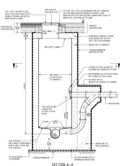
SECTION A-A WITH COVER DETAIL FOR PAVED/ROAD SURFACE
