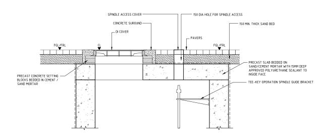
SECTION A - A SLAB FINISH IN PAVED WALKWAY AREAS (OPTIONAL SPINDLE ACCESS)
